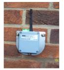
And then we add the tilt sensors. Measuring fine rotational movements and producing high value graphs taking readings every hour. We should start to see changes related to root activity in a few months time.
